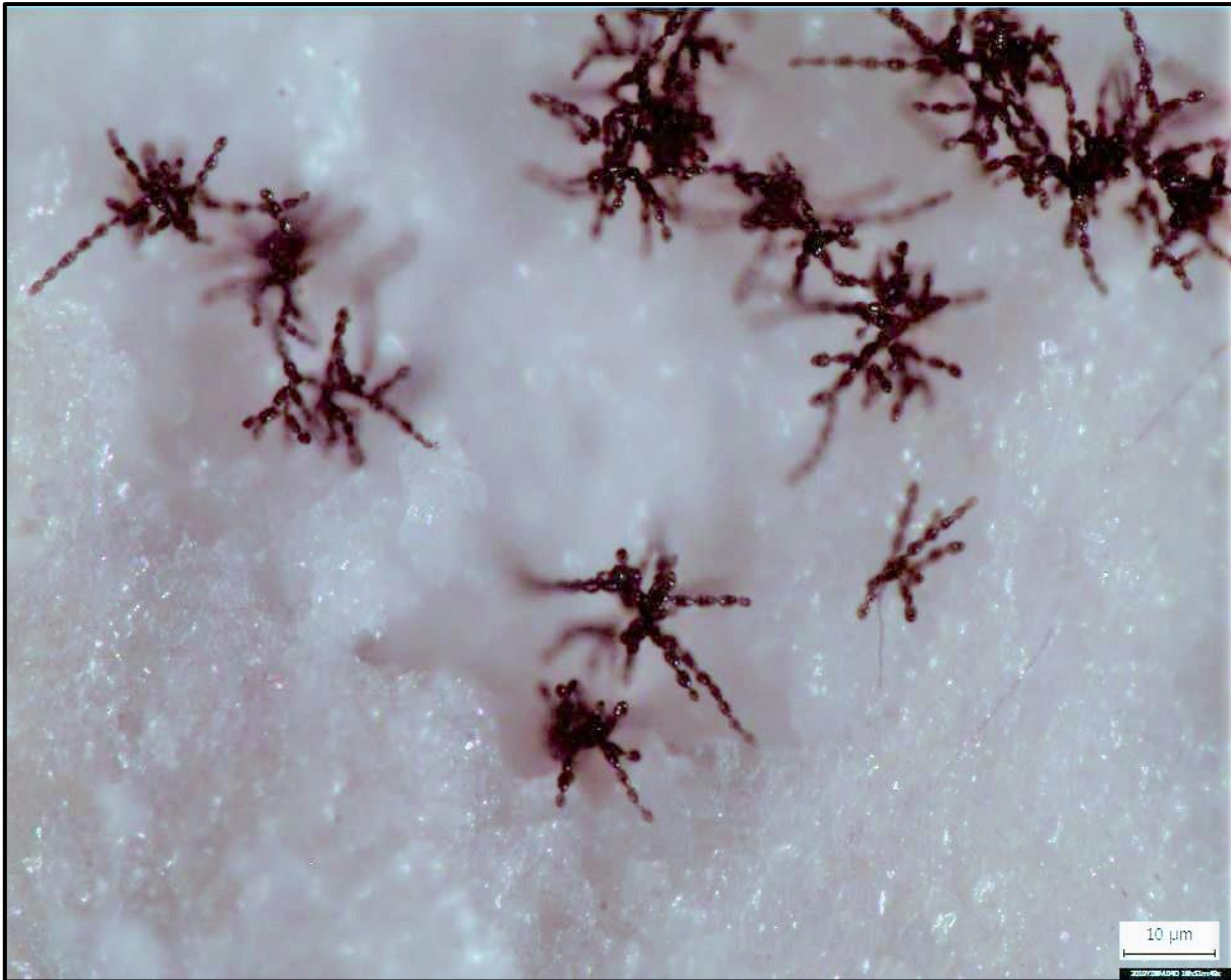
Figure 3, Microscopic image of mould growing on plaster sample at 7.2x magnification on a Nikon AZ100 microscope. The roundish shapes on the mould are conidia. Each conidium can spawn a new colony of mould.
