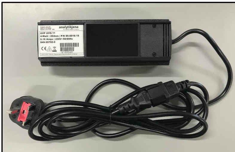
Figure 21, The Analytik Jena 95-0016-15 handheld UV-C lamp. The lamp is often used for sterilisation in small applications as well as forensic document examination and DNA analysis. The lamp was selected for the study because of the strength of the bulb, its portability, and relatively low cost (Analytik Jena, 2019).
