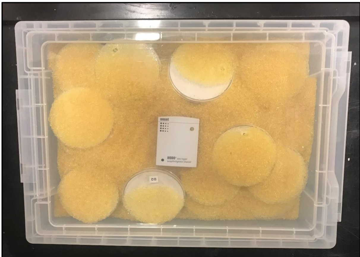
Figure 19, Desiccation of samples in small plastic container with indicating silica gel and datalogger.
