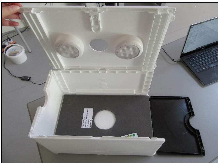
Figure 15, Custom enclosed light box for photography. Contains marked template to hold petri dishes in place, neutral coloured lighting with remote control, and a hole in the top for the camera lens.
