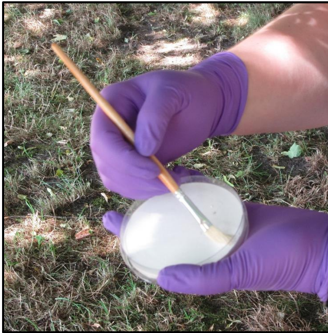
Figure 20, Dry brushing plaster samples with mould growth.
