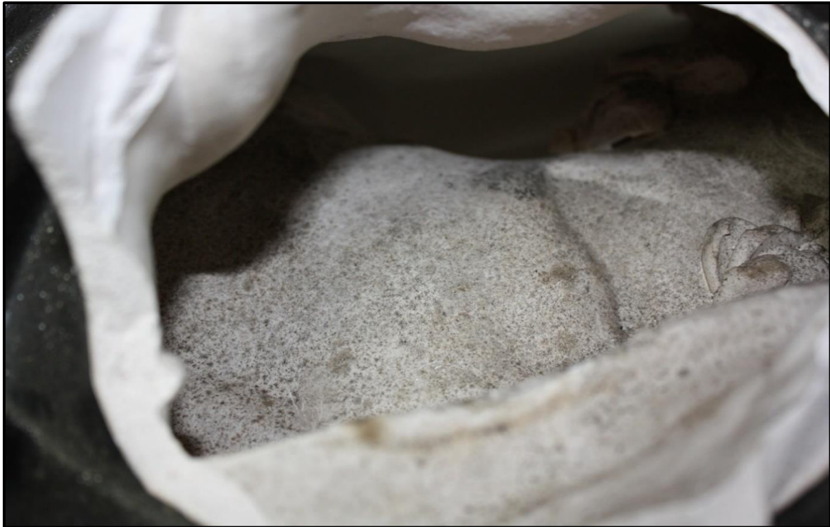
Figure 2, Interior view of main cavity of hollow plaster bust with significant mould growth.
