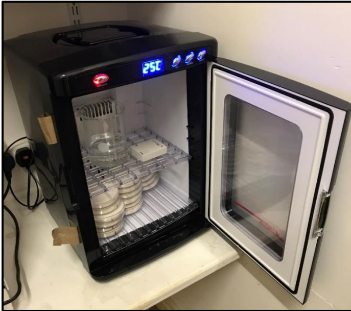
Figure 14, Incubator set-up with inoculated petri dishes, glass beaker of sodium carbonate solution, and datalogger.
